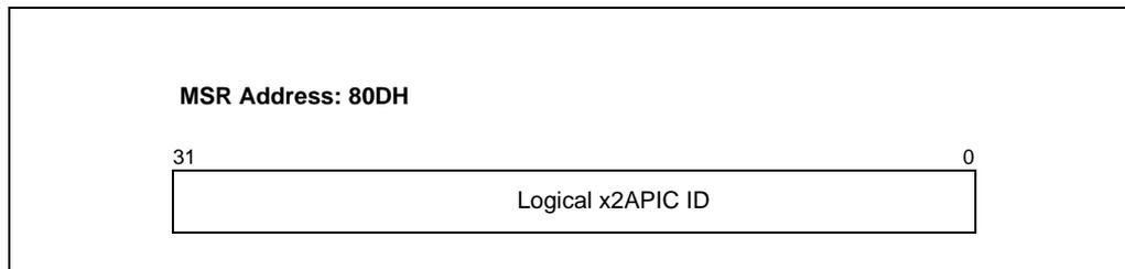
**Figure 2-4. Logical Destination Register in x2APIC Mode**
