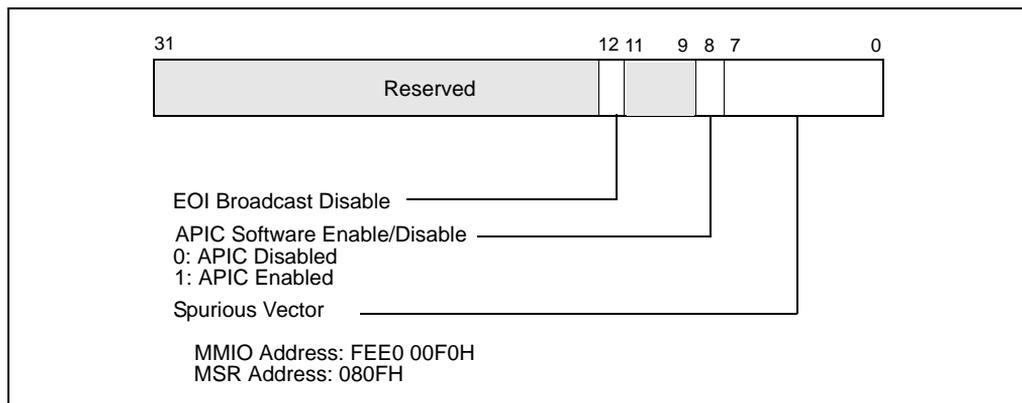
**Figure 2-7. Spurious Interrupt Vector Register (SVR) of x2APIC**
